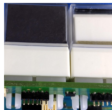
Optional socket mounted on reverse of PCB
