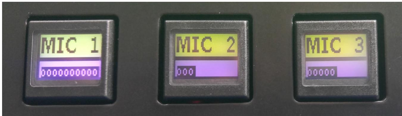
Multi-Segment Color MSC™ allows you to use color, for example, for grouping switches with similar functions (same color in upper segment) and, at the same time, provide operating status information via a different color in the lower segment of the LCD.
