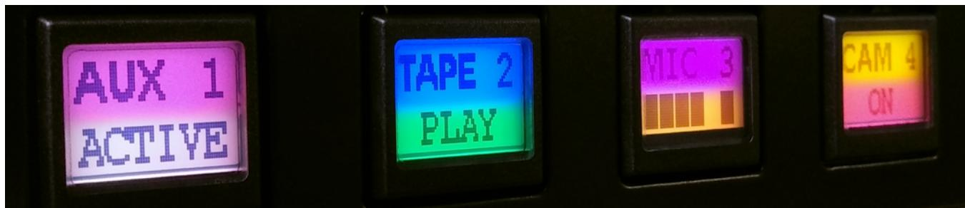
The SE6432 switches introduce Multi-Segment Color MSC™ by allowing different backlight colors in the upper and lower segment of the LCD. For the MSC™ command and an example see pages 18 and 21 respectively.
